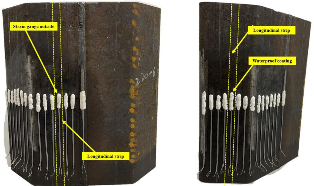
(a) Test arrangement of the outer strain gauges
