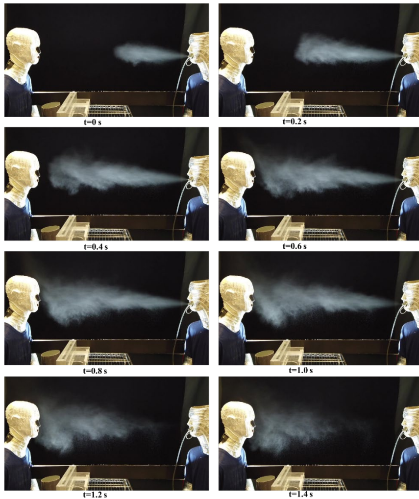
Figure 8 Visualization of interaction between cough jet and PV at a flow rate of 27 L/s
