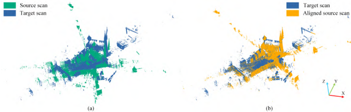
Figure 15: Registration result of the Bremen dataset using GRPC. (a) Source and target point clouds shown in the same coordinate frame. (b) Aligned source and target point clouds.
