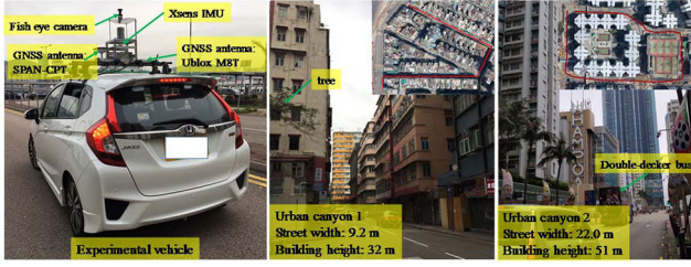
Fig. 5 Experimental vehicle and sensor setup in the left figure. Test scenarios of urban canyons 1 and 2
