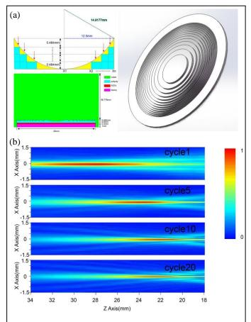
Fig.1 a)The designed specification of the Fresnel lens-focused ultrasonic transducer. b)the focal depth was determined from the acoustic pressure patterns by PZFlex simulaiton
