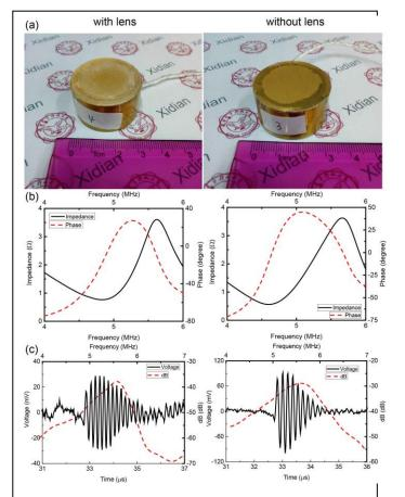
Fig.2 a)the transducer with and without Fresnel lens; b) the frequency dependence of electrical impedance and phase plots of the transducers with and without Fresnel lens; c) the measured pulse-echo waveform with normalized frequency spectrum.
