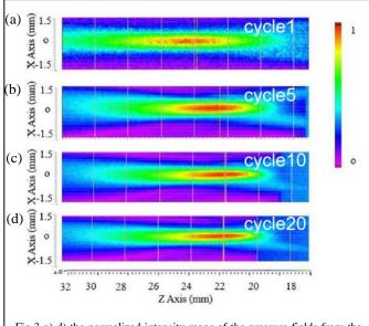
Fig.3 a)-d) the normalized intensity maps of the pressure fields from the Fresnel lens-focused transducer with different cycle numbers of excited signal.
