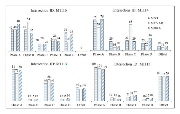
Figure 8: Signal plans from different designing methods (values are in seconds)
