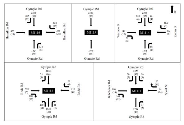
Figure 4: Mean traffic demand in vehicles/hr and standard deviation (values in brackets) on arterial traffic corridor
