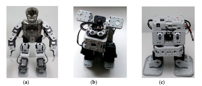
Figure 1. Robotis Bioloids: (http://www.robotis.us/robotis-premium/) Humanoid (a), Puppy (b), and Droid (c).
