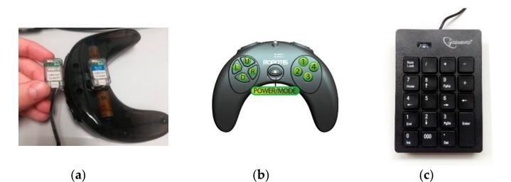
Figure 5. Wireless Bluetooth receiver (a), wireless controller (b), and number pad (c).
