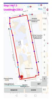
**FIGURE 14.** Demonstration of the ground truth and lamppost position installed with iBeacon on the developed system.
