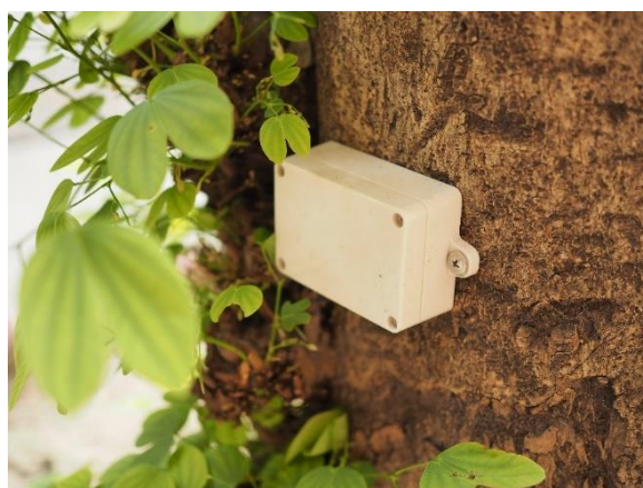
Figure 7. A prototype of a smart sensing technology (SST) sensor. It integrates high-precision accelerometers, geomagnetic sensors, and high-performance microprocessors to measure tree tilt in the urban areas of Hong Kong.
