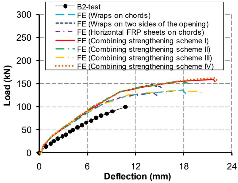
Figure 18. Combination of the strengthening schemes
