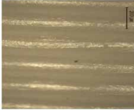
FIGURE 7 Optical micrograph showing the vertical wall surface produced with layer-by-layer deposition of a polymer with a layer thickness of 200 μm.
