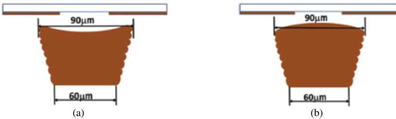
FIGURE 8 Schematic diagrams showing the predicted negative side wall shaped microstructures resulting from deposition in the same place repeatedly and changing the target-substrate distance slowly when deposited (a) in a vacuum and (b) in an inert gas environment.
