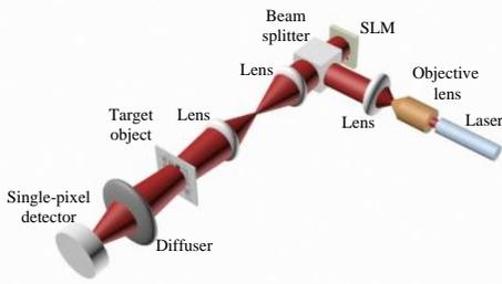
Fig. 5. Schematic of SPI experiment setup for imaging through scattering media.
