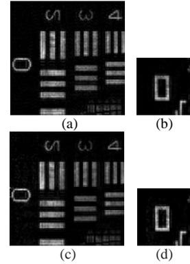
Fig. 4. Experimental comparisons between conventional differential Hadamard method and the proposed method. (a) and (b) the reconstructed objects with size of  $256 \times 256$  and  $128 \times 128$  obtained by using conventional differential Hadamard method. (c) and (d) the reconstructed objects with size of  $256 \times 256$  and  $128 \times 128$  obtained by using the proposed method.
