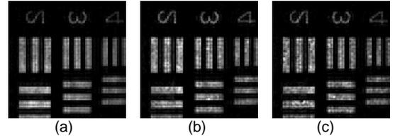
Fig. 6. Object reconstruction in scattering environment by using the proposed method. (a), (b) and (c) reconstructed objects obtained when diffuser model of DG10-600, DG10-220 and DG10-120 is used in the SPI setup, respectively.
