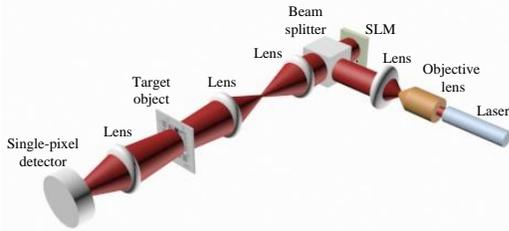
Fig. 2. Schematic of SPI experiment setup: SLM, spatial light modulator.
