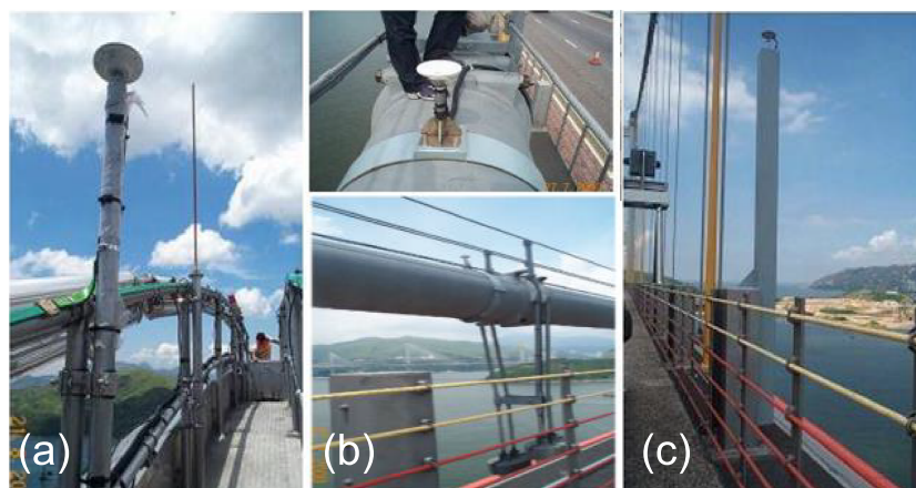
FIGURE 3 GPS receivers deployed at different portions of the bridge: (a) tower top; (b) main cable; (c) deck
