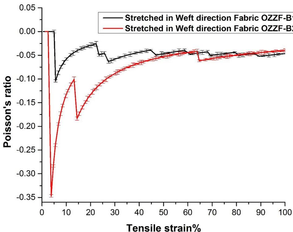
Figure 19. Poisson's ratio versus tensile strain curves of fabrics with two different weft yarn arrangements when stretched along weft direction.
