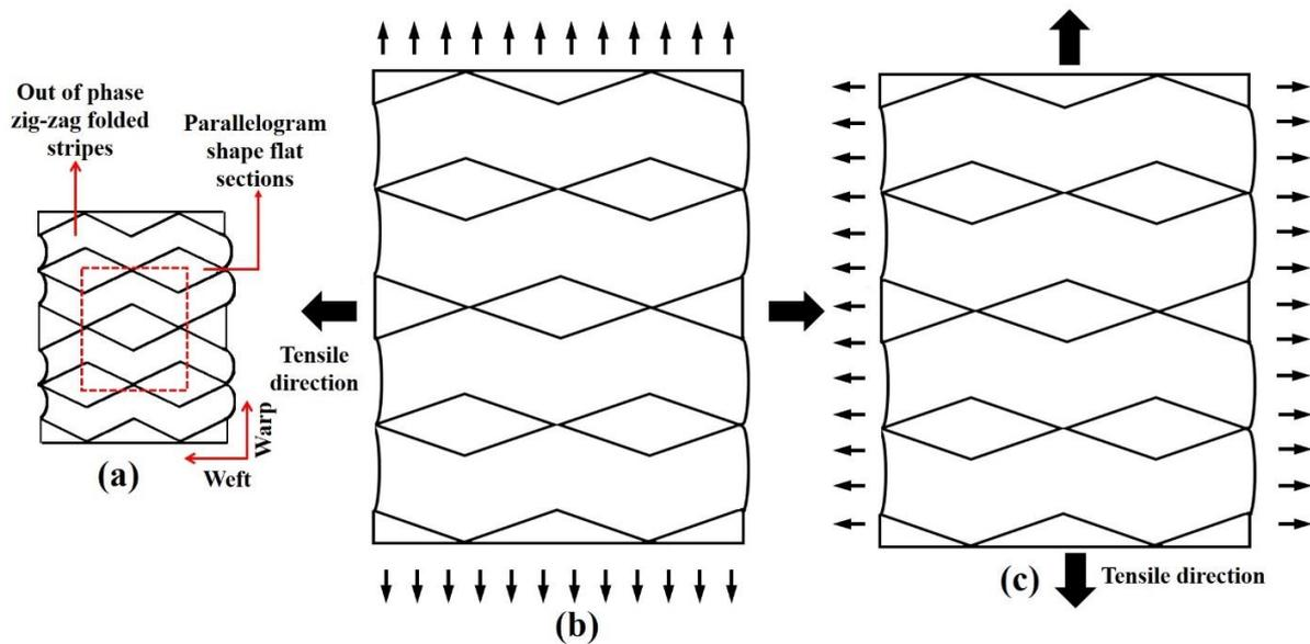
Figure 2. Foldable geometry with parallel out of phase zig-zag folded stripes used for single layered fabric: (a) unstretched state; (b) stretched along weft direction; (c) stretched along warp direction.
