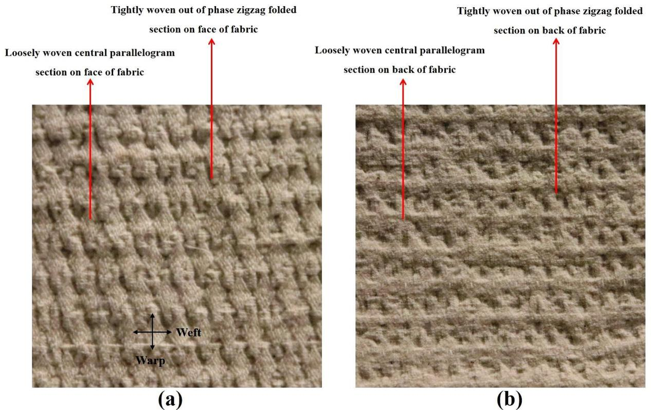
Figure 8. Single layered fabric OZZF-A1: (a) fabric face; (b) fabric back.
