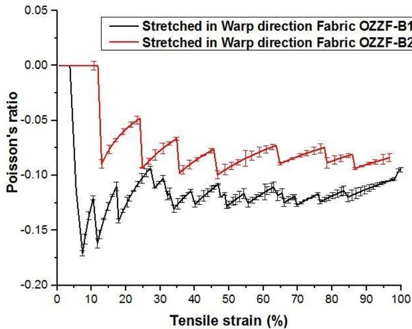
Figure 17. Poisson's ratio versus tensile strain curves of fabrics with two different weft yarn arrangements when stretched along warp direction.
