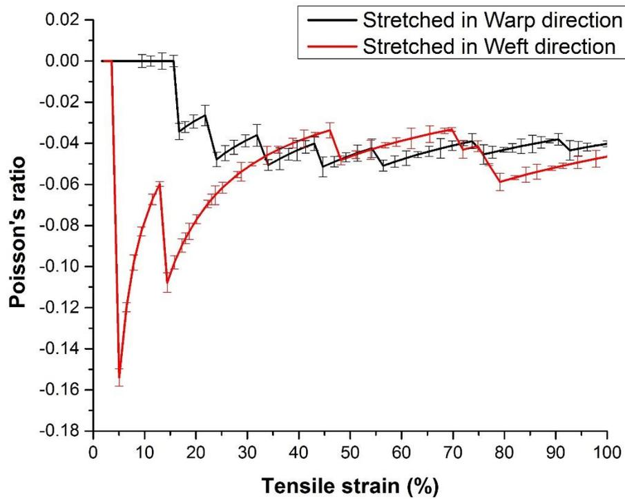
Figure 7. Poisson's ratio versus tensile strain curves of fabric IZZF-2
