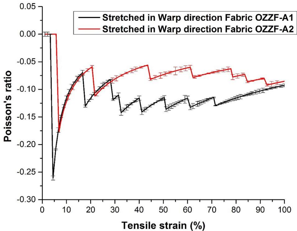
Figure 16. Poisson's ratio versus tensile strain curves of fabrics with two different weft yarn arrangements when stretched along warp direction.
