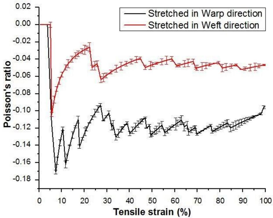
Figure 11. Poisson's ratio versus tensile strain curves of fabric OZZF-B1.
