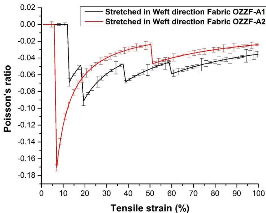
Figure 18. Poisson's ratio versus tensile strain curves of fabrics with two different weft yarn arrangements when stretched along weft direction.
