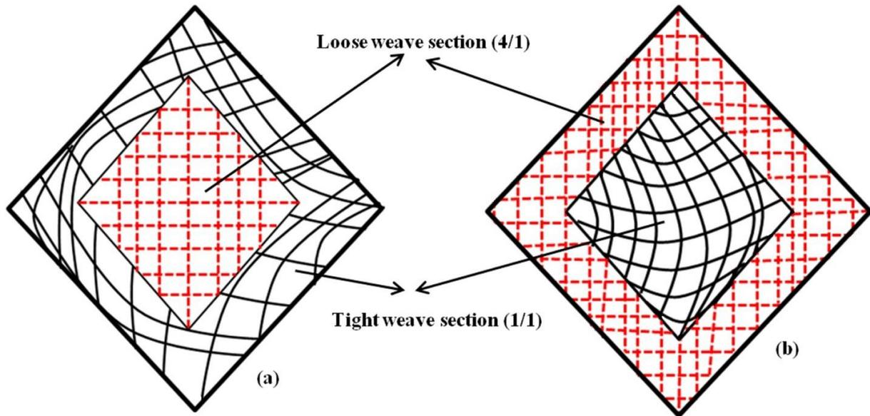
Figure 15. Illustration of loose weave and tight weave placement: (a) OZZF-A1; (b) OZZF-B1.
