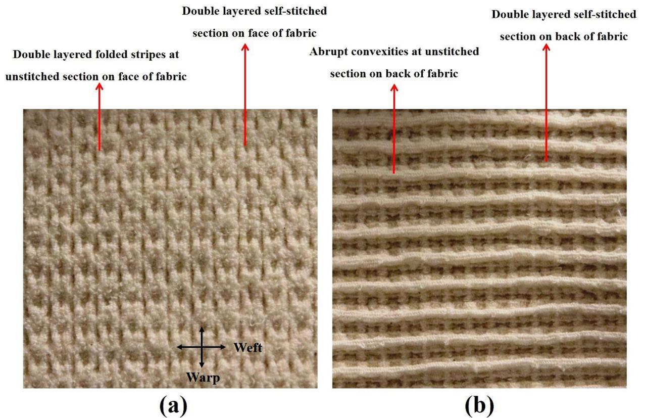
Figure 6. Double layered fabric (IZZF2) with parallel in-phase zig-zag folds: (a) fabric face; (b) fabric back.
