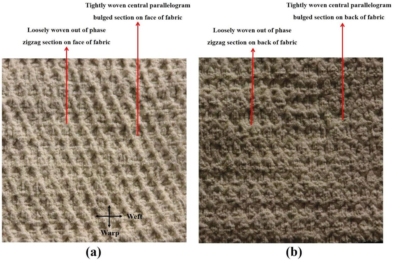
Figure 9. Single layered fabric OZZF-B1: (a) fabric face; (b) fabric back.
