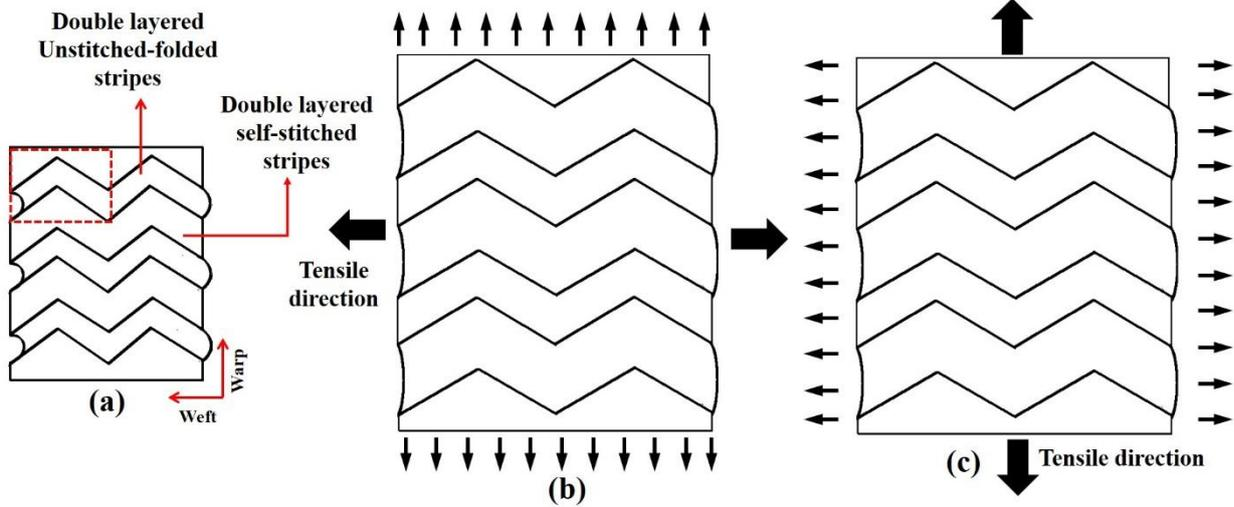
Figure 1. Foldable geometry with parallel in phase zig-zag stripes used for double layered fabric: (a) unstretched state; (b) stretched along weft direction; (c) stretched along warp direction.
