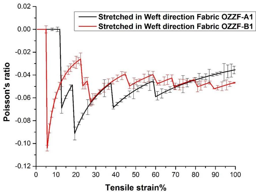
Figure 14. Poisson's ratio versus tensile strain curves of fabrics when stretched along weft direction.
