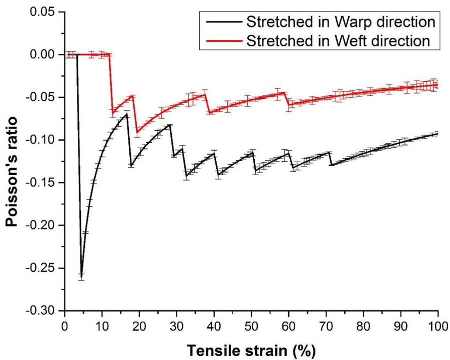
Figure 10. Poisson's ratio versus tensile strain curves of fabric OZZF-A1.
