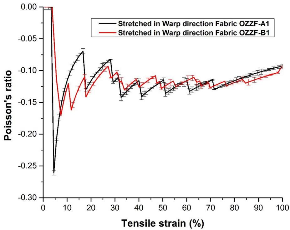
Figure 13. Poisson's ratio versus tensile strain curves of fabrics when stretched along warp direction.
