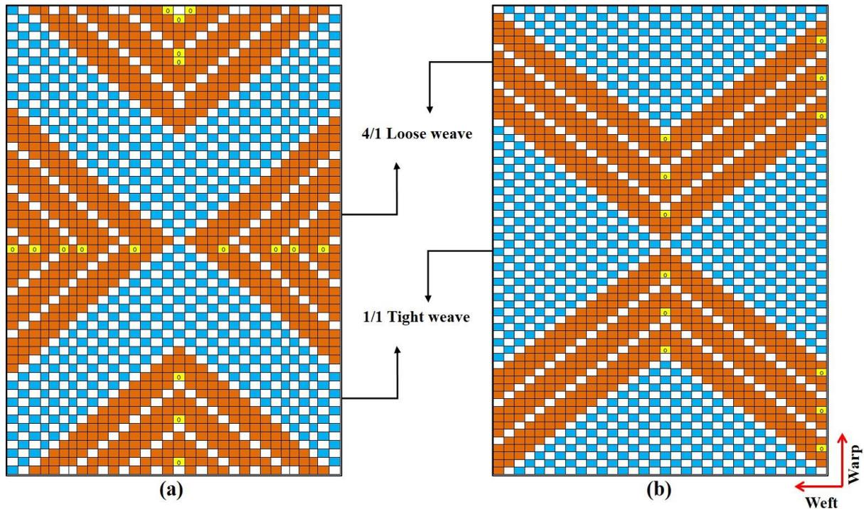
Figure 5. Interlacement patterns of single layered fabrics: (a) fabric with out of phase folded stripes OZZF-A1 and OZZF-A2; (b) fabric with out of phase flat stripes OZZF-B1 AND OZZF-B2.
