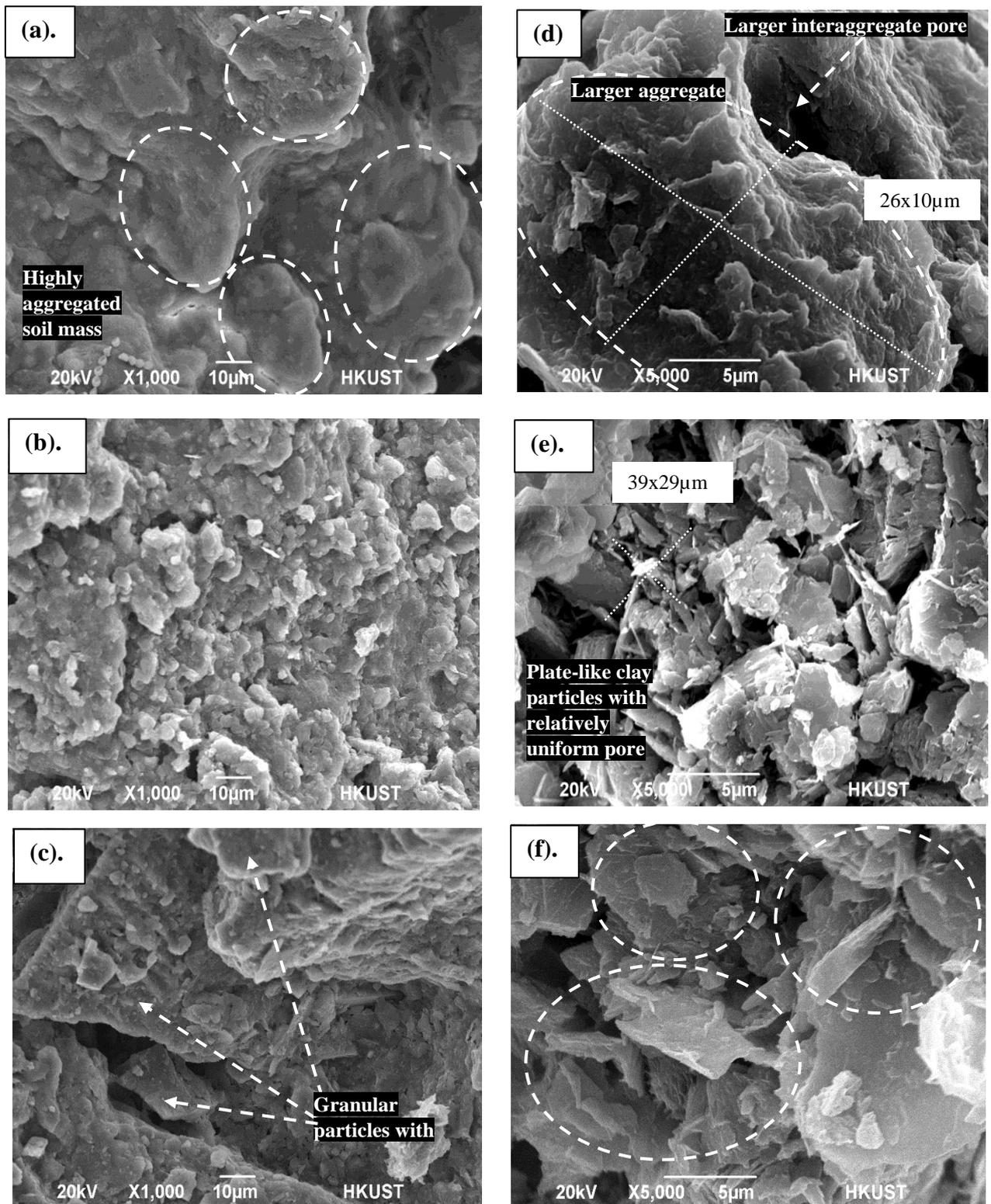
**Figure 9: SEM images of the three soils at different magnifications; (a) LAT under X 1,000; (b) CDV under X 1,000; (c) CDG under X 1,000; (d) LAT under X 5,000; (e) CDV under X 5,000; (f) CDG under X 5,000.**
