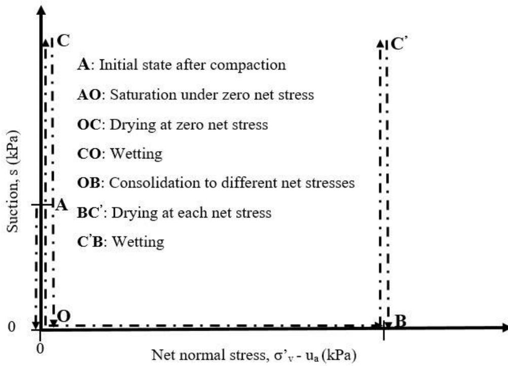
Figure 4: Stress paths for measuring drying - wetting water retention behaviour.
