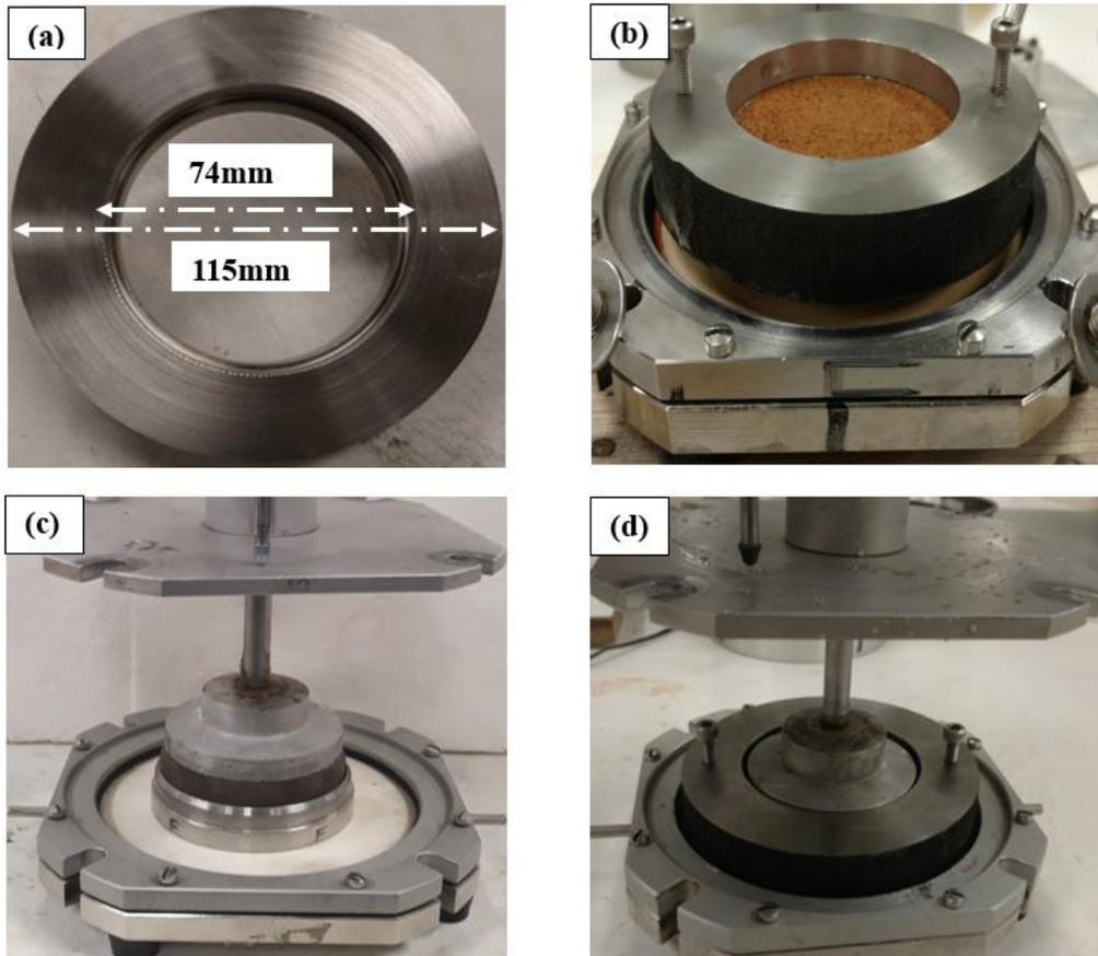
**Figure 3: Guard cell developed to eliminate eccentric loading of specimen. (a) Newly fabricated guard cell; (b) Lateral view of mounted guard cell; (c) Configuration of specimen inside the setup without the guard cell; (d) Configuration of specimen inside the setup with the guard cell.**
