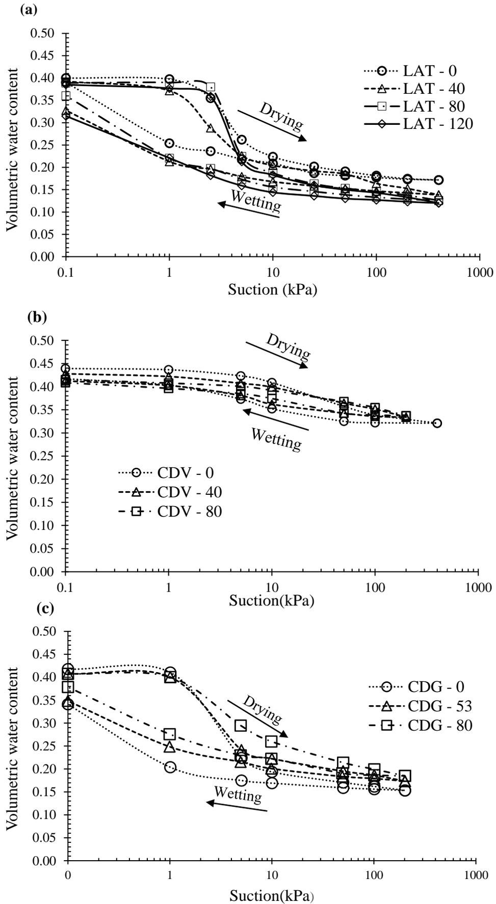
**Figure 5: SDSWRC in terms of volumetric water content against suction under different net stresses; (a) for LAT; (b) for CDV; (c) for CDG.**
