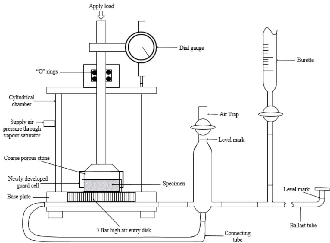
**Figure 2: Schematic diagram of improved stress-controlled pressure plate apparatus (after Ng & Pang, 2000)**
