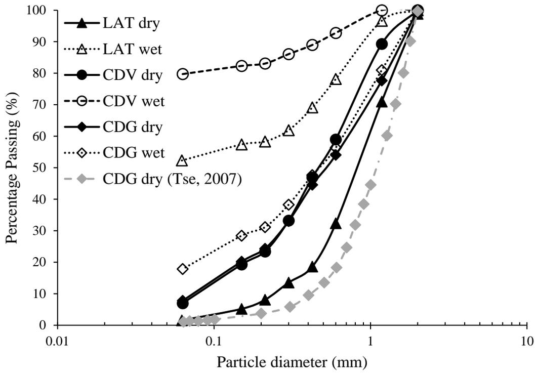
**Figure 1: Particle size distribution of the soils studied.**
