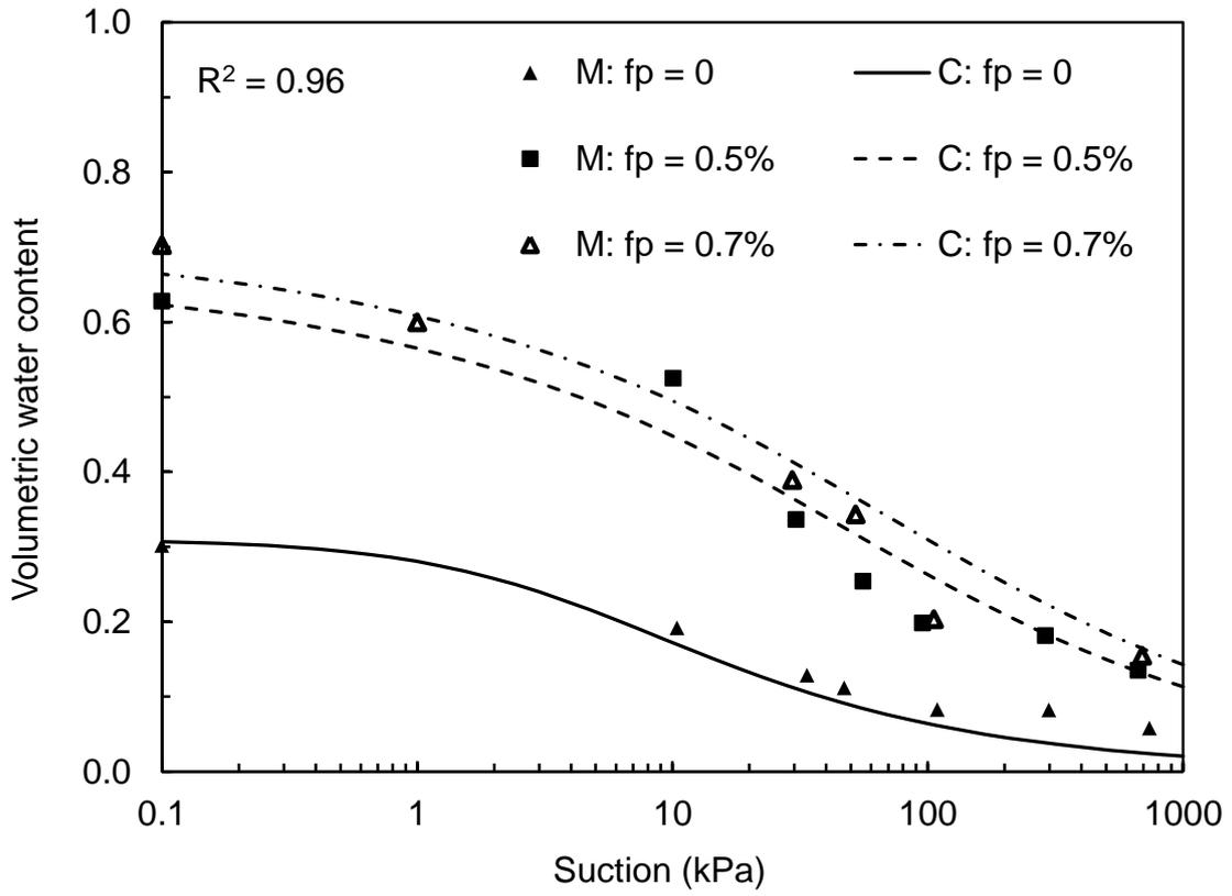
Figure 9. Measured (M) (Narjary et al., 2012) and calculated (C) water retention curves of a sand containing biopolymer-based Pusa hydrogel
