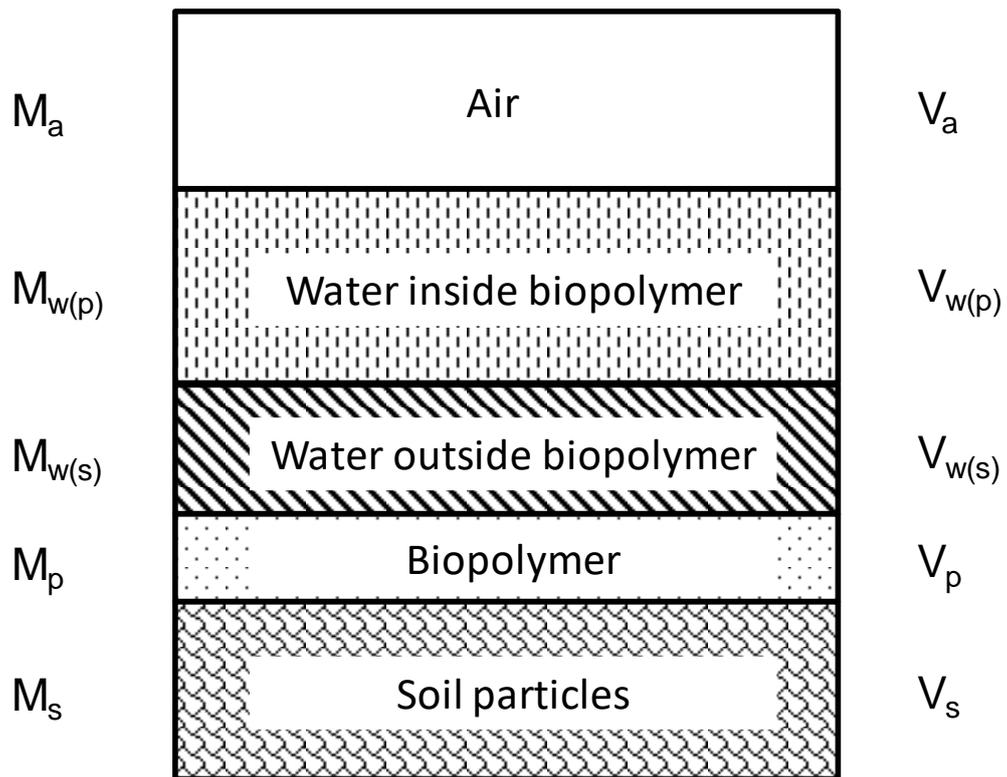
Figure 2. Phase diagram of a soil containing biopolymer
