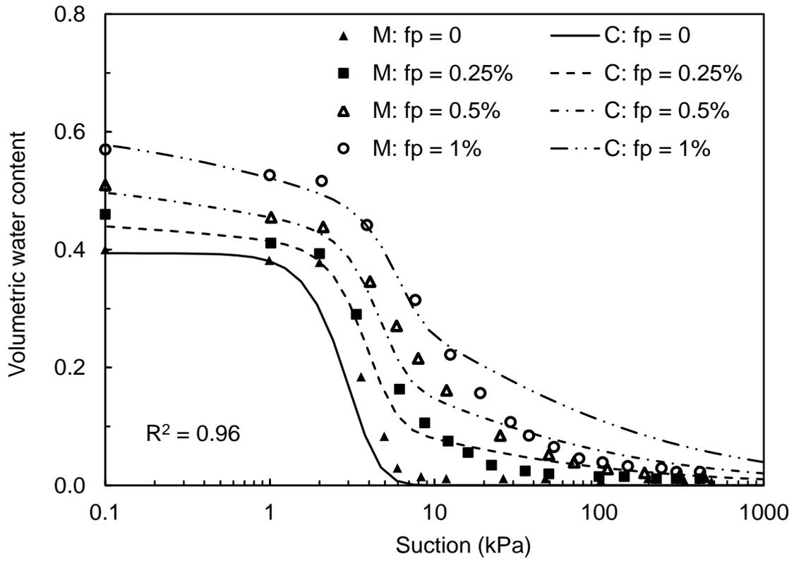
Figure 8. Measured (M) (Rosenzweig et al., 2012) and calculated (C) water retention curves of a Chromic Luvisol containing xanthan gum
