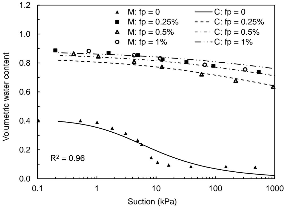
Figure 12. Measured (M) (Tran et al., 2018) and calculated (C) water retention curves of a sand containing xanthan gum
