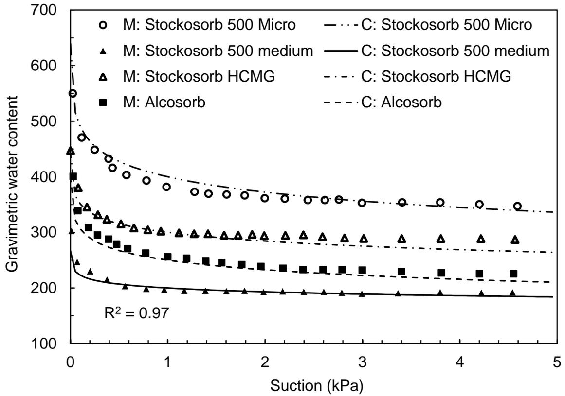
Figure 3. The relationship between gravimetric water content and suction for various pure biopolymers (M and C denote measured and calculated results, respectively; the test data was reported by Bhardwaj et al., 2007)
