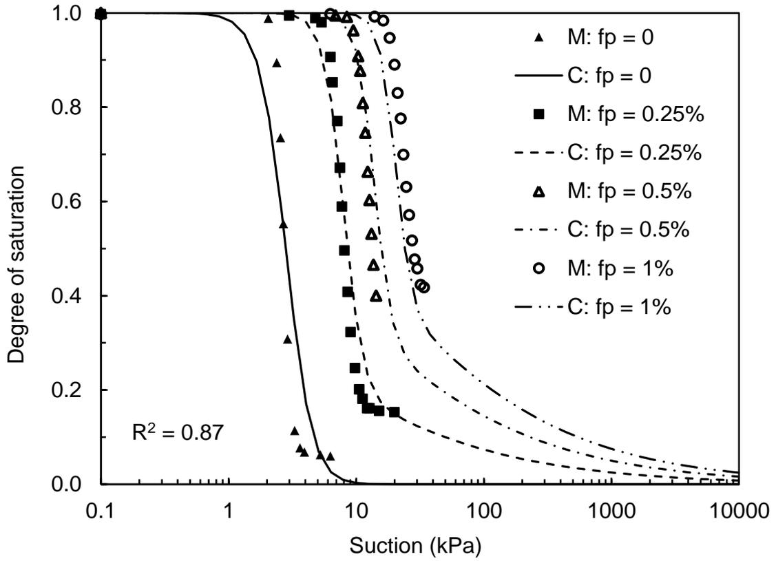
Figure 11. Measured (M) (Jung et al., 2017) and calculated (C) water retention curves of a sand containing polymer produced by acrylamide
