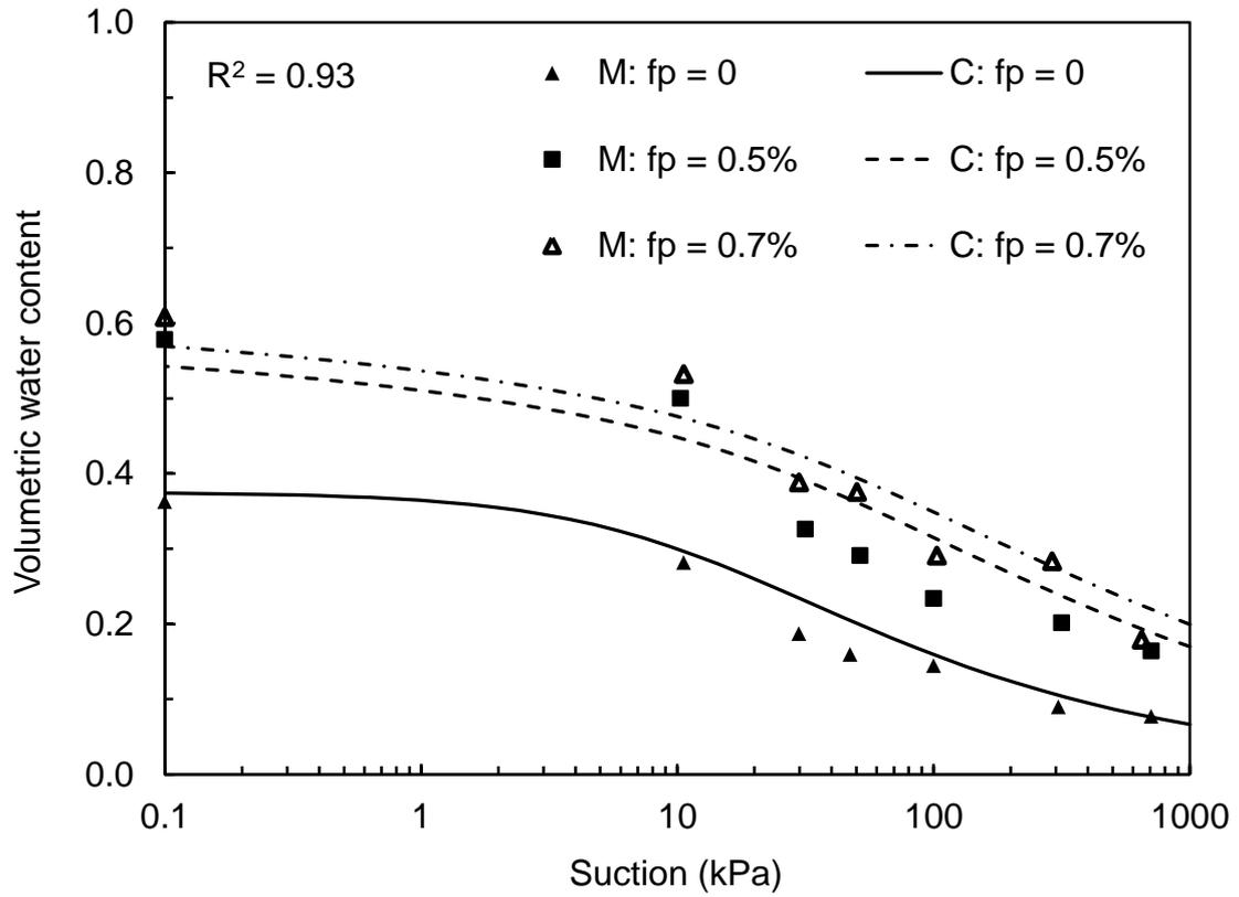
Figure 10. Measured (M) (Narjary et al., 2012) and calculated (C) water retention curves of a sandy loam soil containing biopolymer-based Pusa hydrogel
