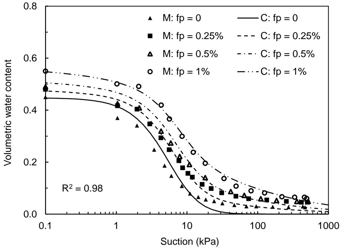
Figure 7. Measured (M) (Rosenzweig et al., 2012) and calculated (C) water retention curves of Caesarea sand containing xanthan gum
