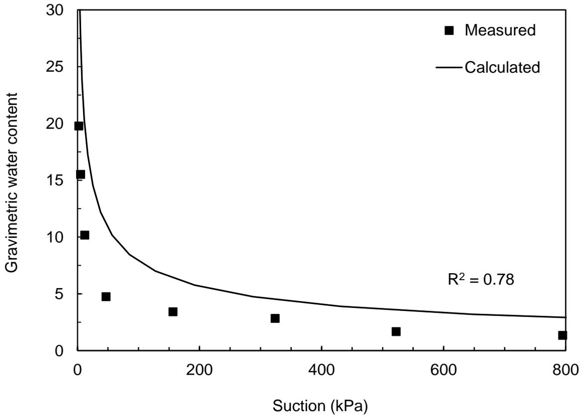
Figure 4. The relationship between gravimetric water content and suction for pure xanthan gum in a wide suction range (the test data was reported by Rosenzweig et al., (2012))
