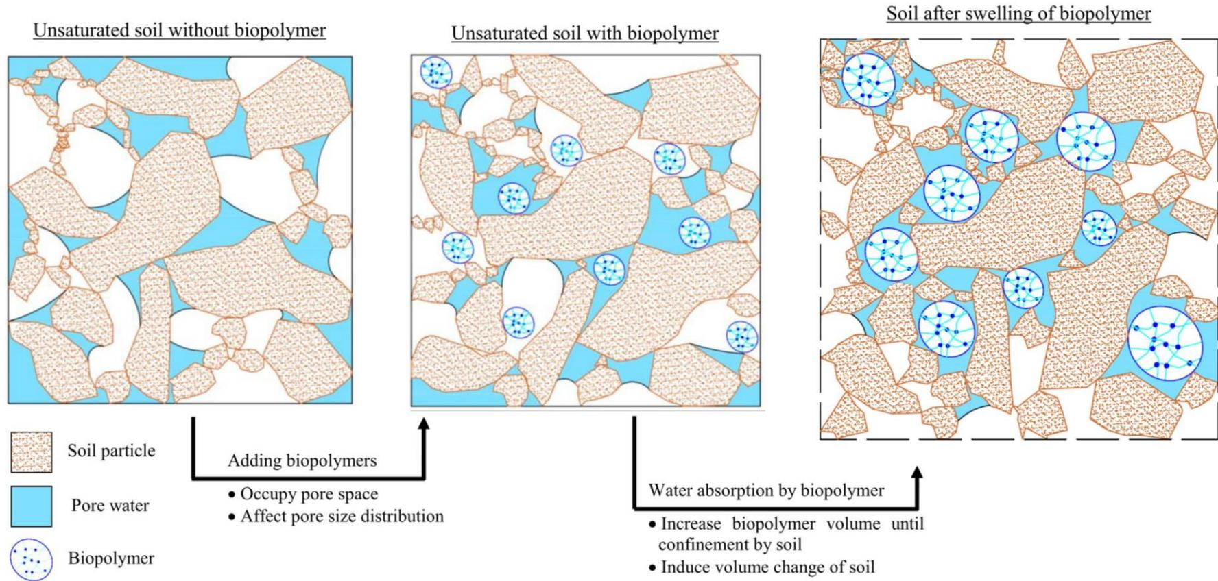
Figure 1. Schematic diagram illustrating biopolymer-soil interactions and the four assumptions made in this study
