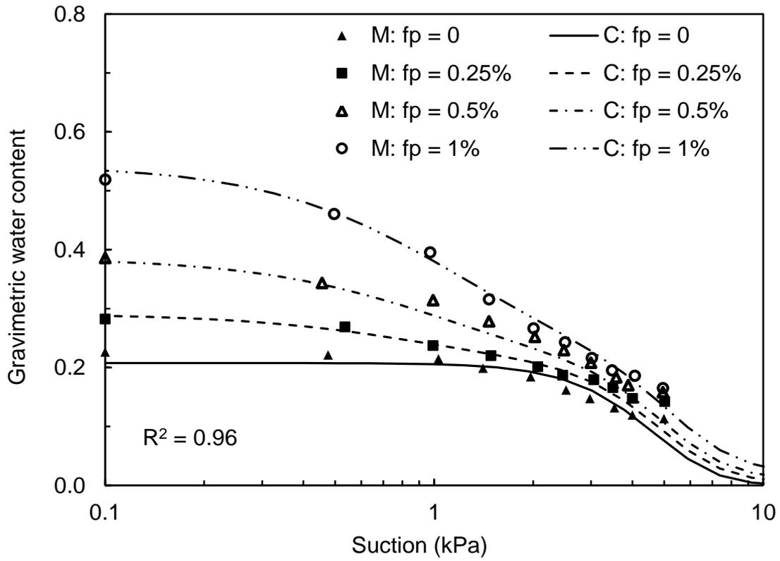
Figure 6. Measured (M) (Bhardwaj et al., 2007) and calculated (C) water retention curves of a sand containing polyacrylamide (PAM)
