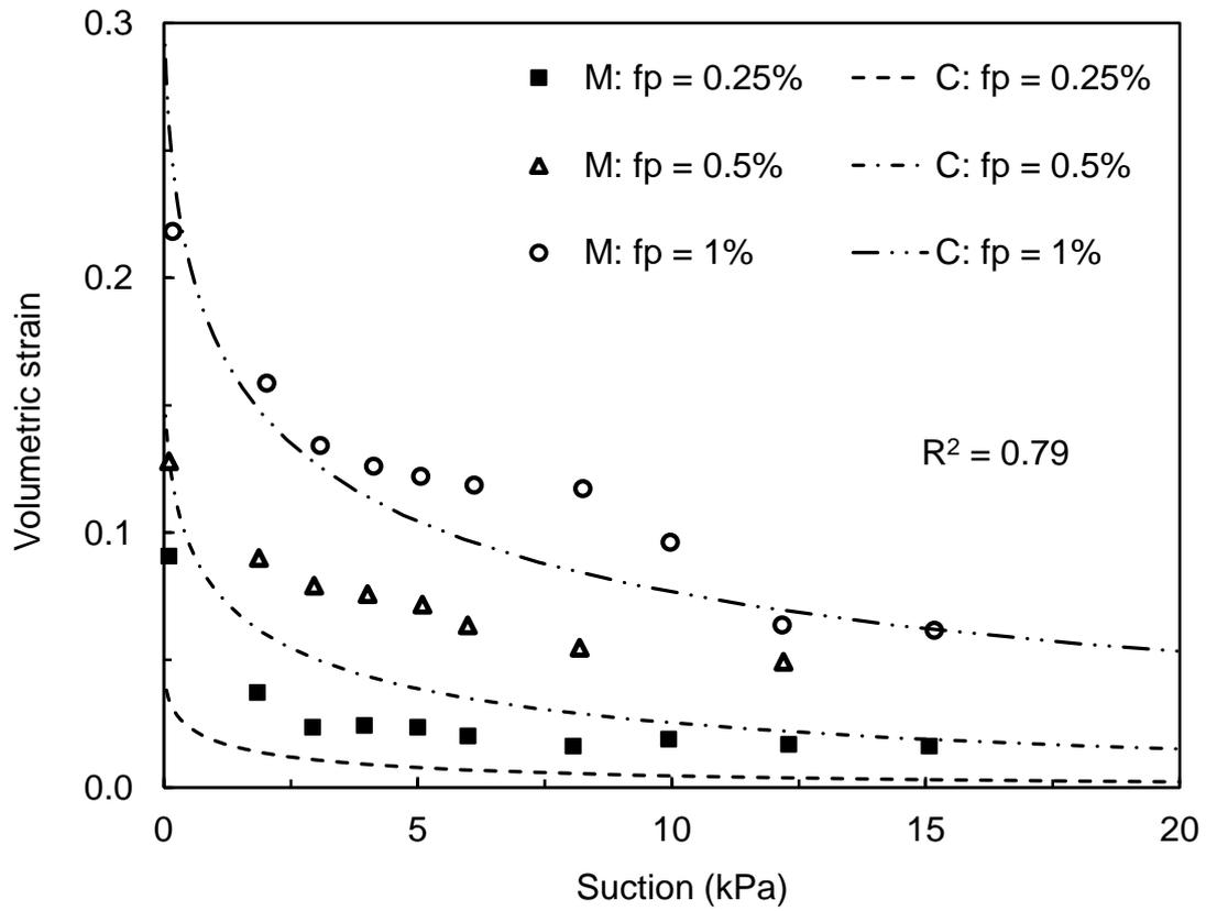
Figure 5. Measured (M) (Rosenzweig et al., 2012) and calculated (C) volumetric strains of a sand induced by the swelling of biopolymer
