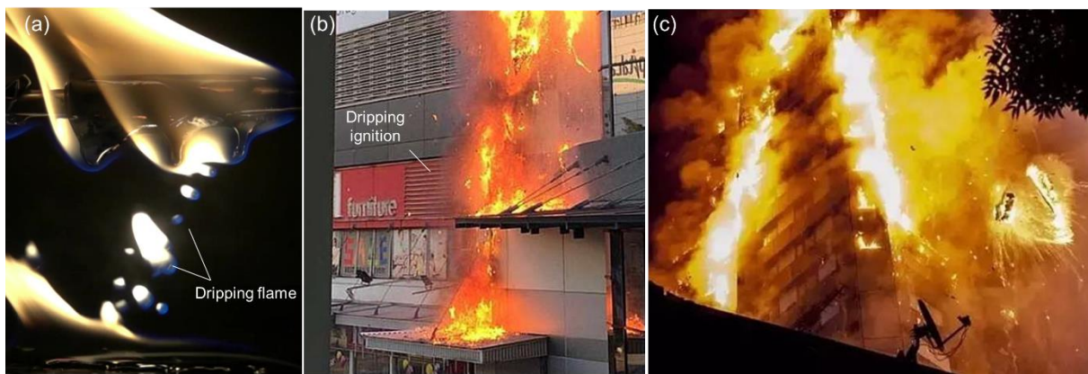
Figure 1. The dripping phenomenon and the resulted ignition process in (a) the electrical wire fire, and (b) a façade fire in China, and (c) Grenfell Tower fire in London [9].
