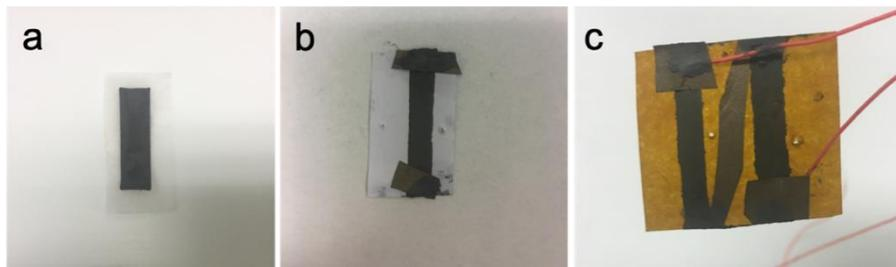
Figure 4. Flexible TE film fabricated on (a) water-soluble paper, (b) typing paper and (c) PI paper. The dimension of these three legs is 30mm\*4mm\*0.05mm.
