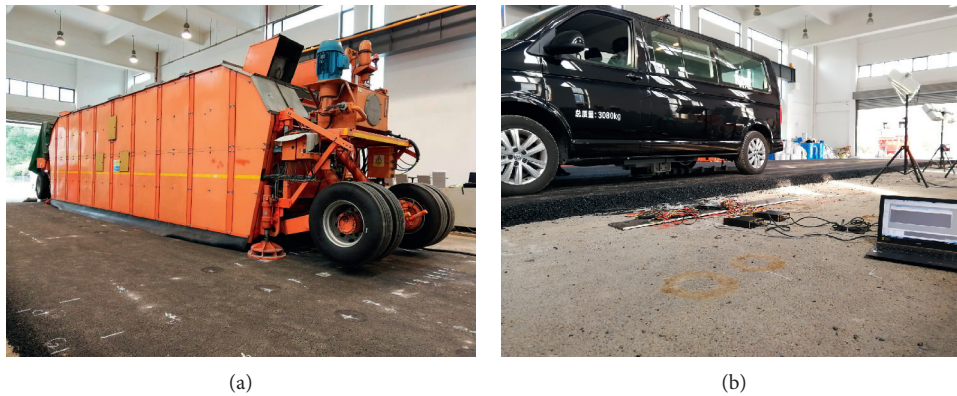
FIGURE 4: The photographs of (a) vehicular loading test and (b) FWD loading test.
