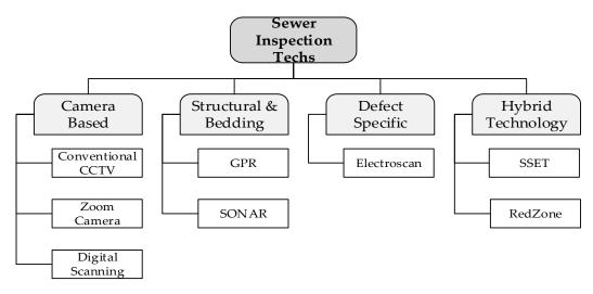
Figure 3. Different sewer pipeline inspection techniques.
