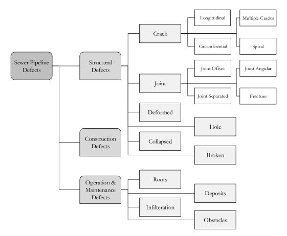
Figure 2. Common sewer pipeline defect classification. Adopted from PACP [7].
