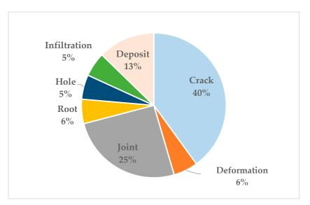
Figure 8. Studies on detection automation of different types of sewer defect.
