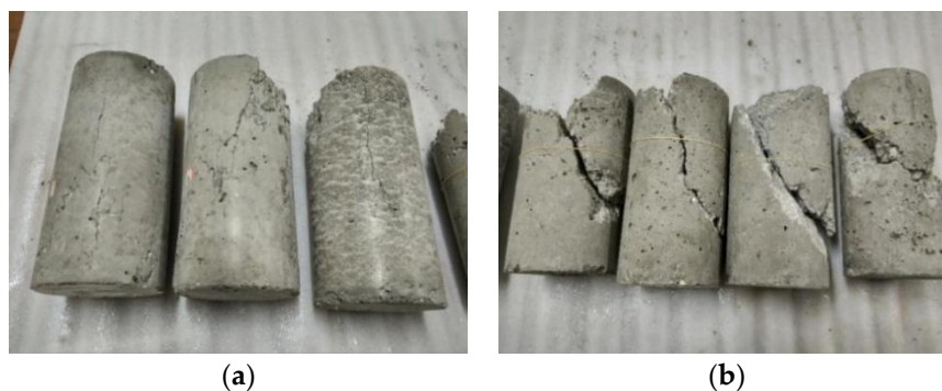
Figure 4. Failure modes: (a) uniaxial compression; (b) triaxial compression (from left to right \sigma_1 = 6, 12, 18, 24 MPa).
