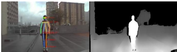
Figure 8. A person stands still while in front of the camera to enable the distance value of the waist to be recorded
