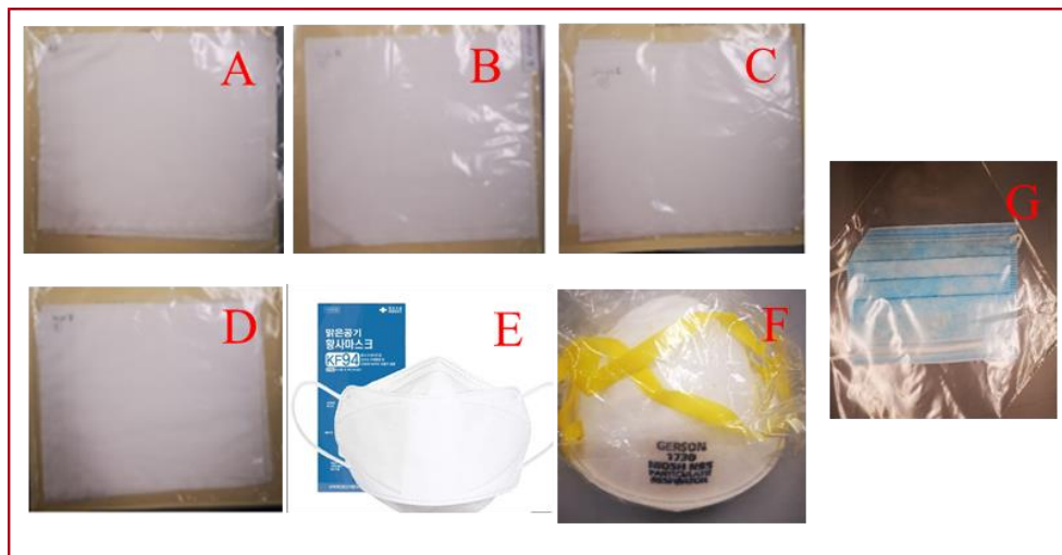
Fig. 2. Mask samples tested in study: (A–D) materials for reusable masks, and (E) KF94, (F) N95 and (G) surgical masks.
