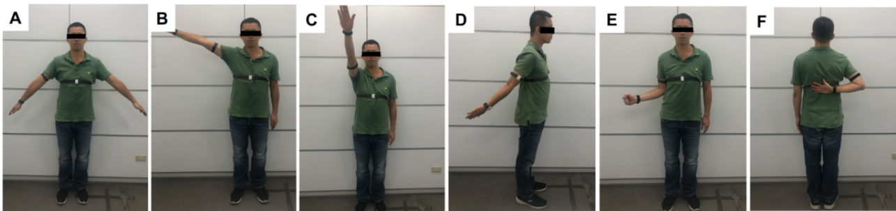
Figure 1. Angular measurement of the shoulder with motion sensors worn on the body for (A) calibration, (B) shoulder abduction, (C) shoulder flexion, (D) shoulder extension, (E) shoulder external rotation, (F) shoulder internal rotation.
