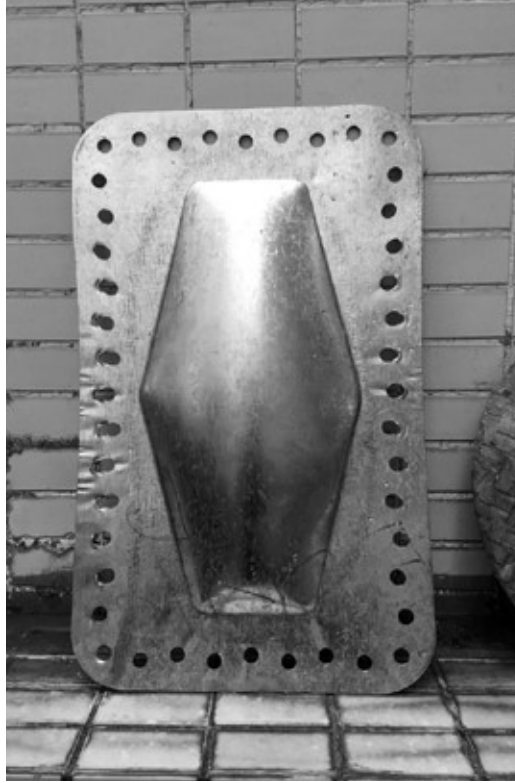
Figure 3 (left): Current pressure forming rig, with a hexagon-shaped forming die. Source: author .
