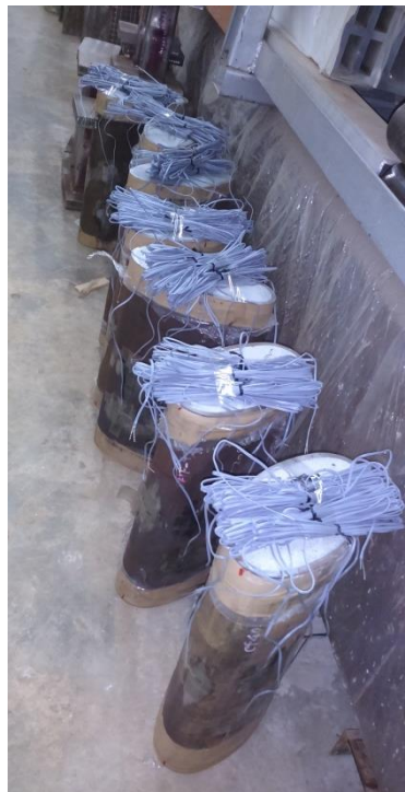
Figure 3: Prepared concrete-filled stub column specimens with strain gauges
