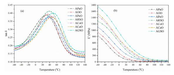
Figure 3. (a) Loss factor and (b) storage modulus of the UV-cured films.
