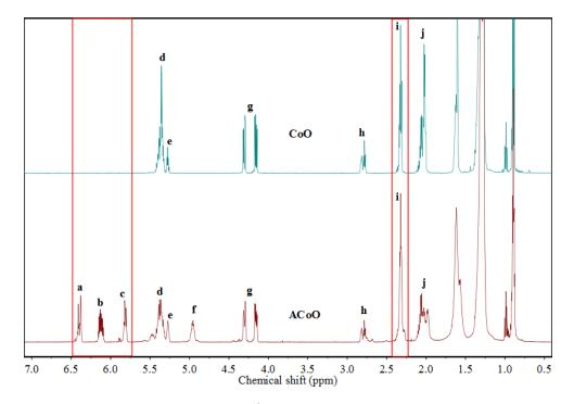
**Figure 2.** Proton nuclear magnetic resonance (<sup>1</sup>H NMR) spectra of CoO and ACoO. Note: The lowercase letters corresponded to the protons in Scheme 2.
