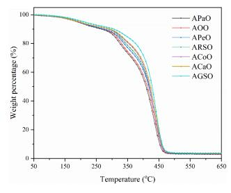
Figure 4. Thermo-gravimetric analysis (TGA) results of the UV-cured films.
