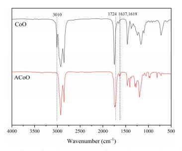
**Figure 1.** Fourier transform infrared (FT-IR) spectra of corn oil (CoO) and corn oil-based acrylate prepolymer (ACoO).
