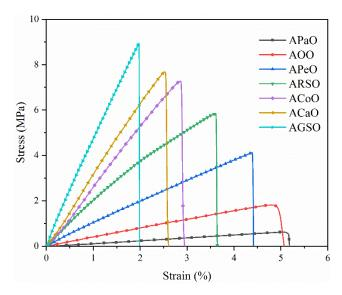
Figure 5. Stress-strain curves of the UV-cured films.
