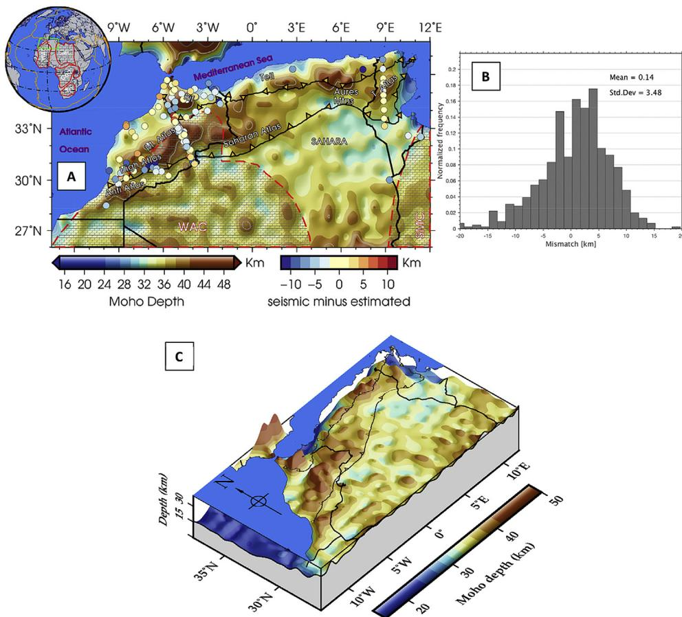
Fig. 7. Regional map of the Moho depth estimated based on a regularized non-linear inversion of the sediment-corrected Bouguer gravity data. The Moho depth differences between seismic and gravimetric solutions is shown at seismic sites. Figure also includes the histogram of these differences.
