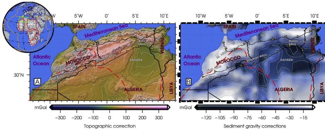
**Fig. 3.** Regional maps of: (A) the topographic-bathymetric and (B) sediment gravity corrections computed on a  $5' \times 5'$  grid of surface points.
