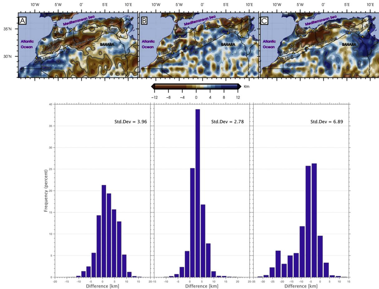
**Fig. 10.** Comparison between regional crustal thickness models and our model. The Moho depth differences with respect to: (A) GEMMA model by Reguzzoni et al. [54], (B) Tugume13 model by Tugume et al. [55], and (C) Tedla11 model by Tedla et al. [56].
