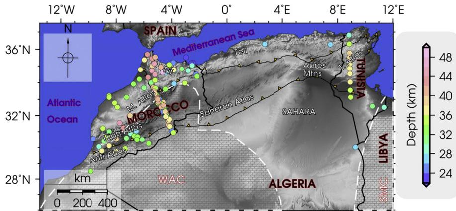
Fig. 5. Seismic Moho depth estimates from receiver functions analysis seismograph stations (circles), superimposed on a regional shaded topography.
