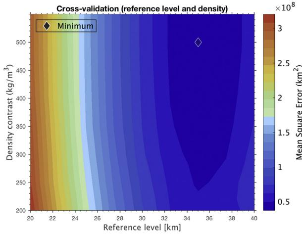
Fig. 6. Validation steps exploited to determine the Moho reference depth and the Moho density contrast. The colour scale represents the Mean Square Error. The best-fit model is marked by a grey rectangular (for the Moho density contrast of 500 kg m<sup>-3</sup> and the Moho reference depth of 35 km).
