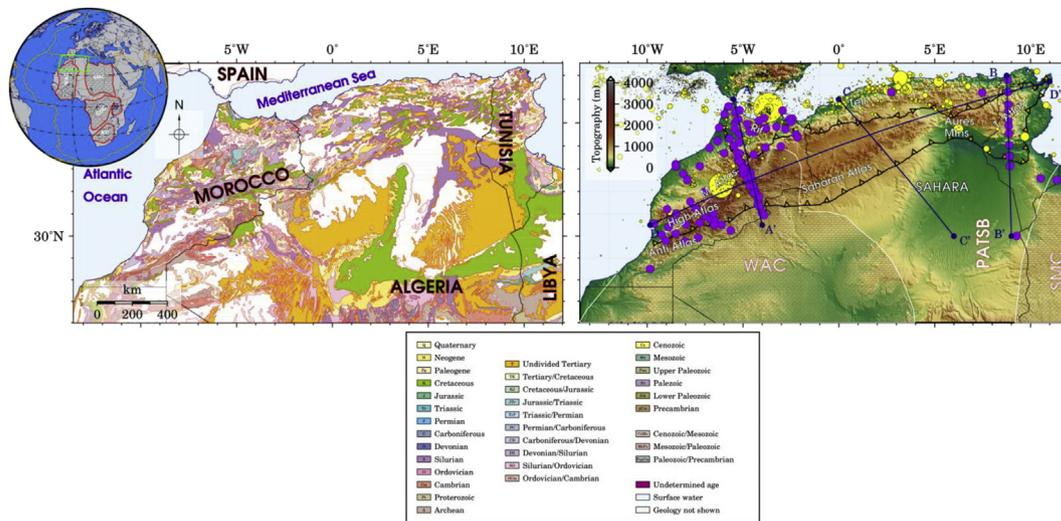
**Fig. 1.** Regional geological and tectonic configuration of the Atlas region including seismicity. AA', BB', CC' and DD' (Fig. 10) indicate four selected profiles. The inset shows the location of the Rif-Tell-Atlas orogenic region along the Eurasian-African plate boundary. The orange lines indicate plate boundaries according to Bird [24]. Notation used: West African Craton (WAC), Pan-African Trans-Saharan Belt (PATSB) and Sahara Meta-Craton (SMC).
