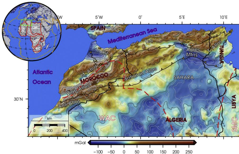
Fig. 2. Regional maps the free-air gravity anomalies computed on a  $5' \times 5'$  grid of surface points.
