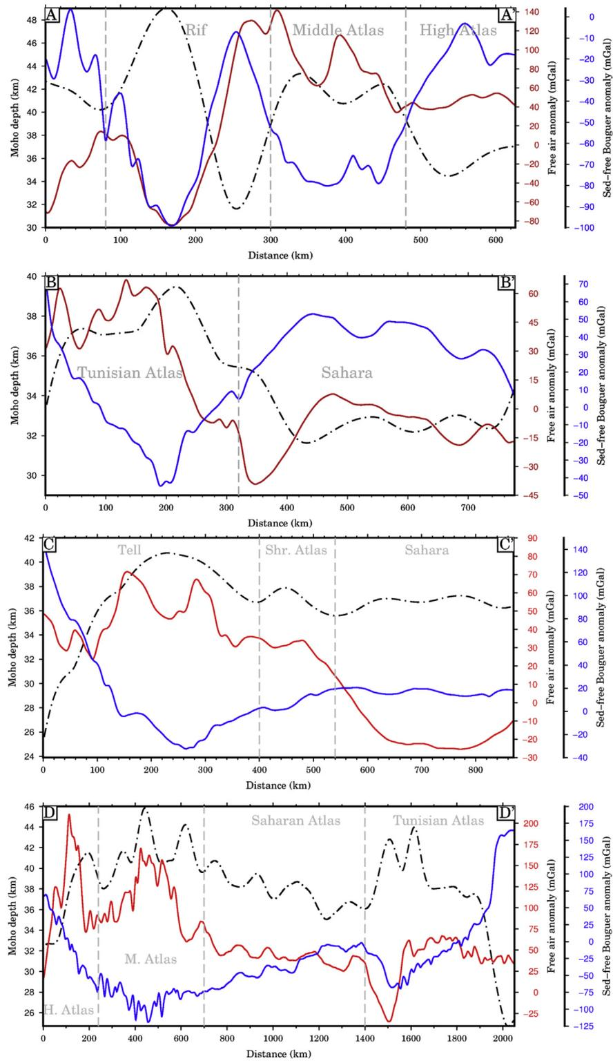
**Fig. 11.** Study profiles for comparing values of the free-air and Bouguer gravity anomalies with the Moho depth and the topography across the Rif-Tell-Atlas orogenic region (see locations in Fig. 1): AA' profile along the Morocco Atlas system, BB' profile along the Tunisia Atlas system, CC' profile along the Atlas system, and DD' profile through Morocco, Algeria, and Tunisia.
