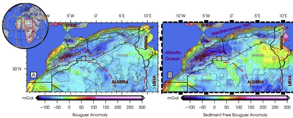
**Fig. 4.** Regional maps of the Bouguer gravity anomalies: (A) before and (B) after applying the sediment gravity correction computed on a  $5' \times 5'$  grid of surface points.
