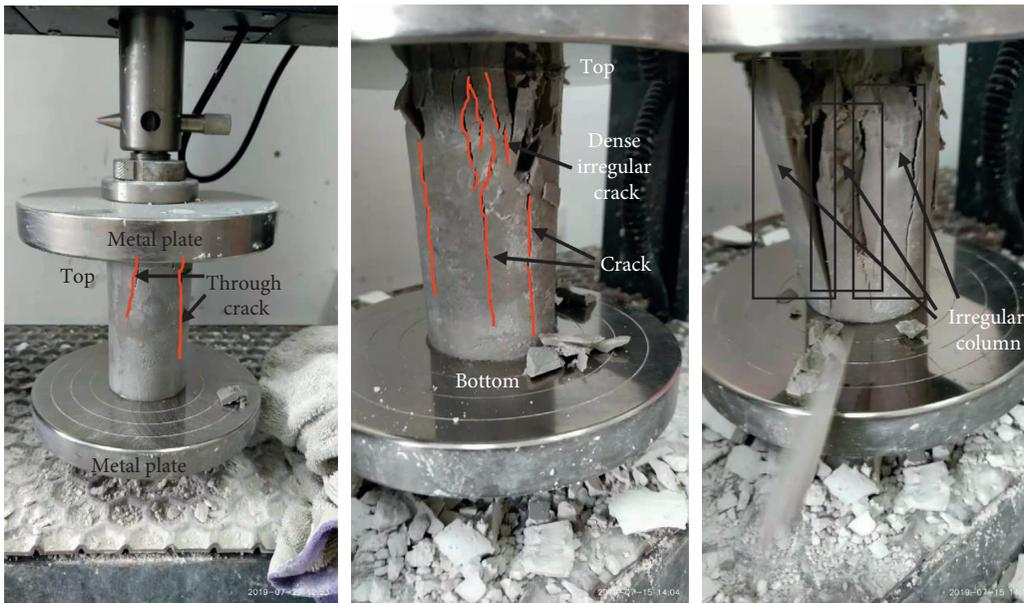
FIGURE 8: Fracture morphology of the cylindrical specimen under compression.
