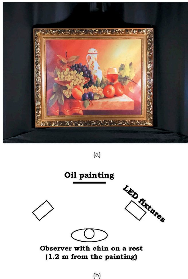
Fig. 1. (a) Photograph of the oil painting under the illumination and (b) schematic layout of the experiment setup (not to scale).
