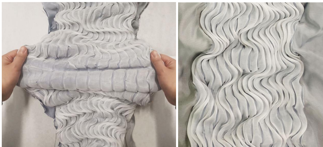
Figure 7. Stretched state (left) and relaxed state(right) of POF sample(h)
