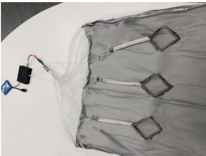
Figure 14. Structure of the touch-sensitive POF fabric (back view).
