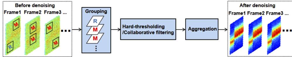
Fig. 1. Flowchart of the proposed VBM3D denoising for BOTDA. “R” and “M” represent the reference blocks and the matched ones.
