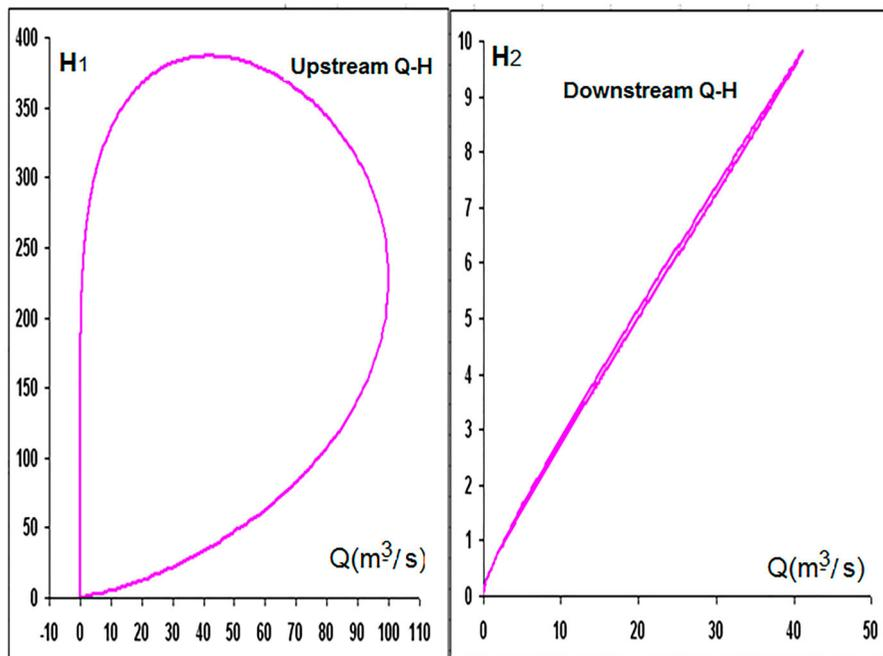
**Figure 4.** Stage-discharge upstream and downstream of detention rockfill dams.
