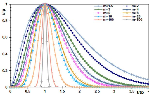
Figure 1. The effects of  $m$  factor on inflow hydrograph shape in dimensionless form.
