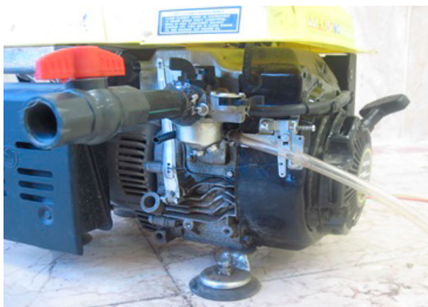
Figure 4. Methane and air inlets to the engine.
