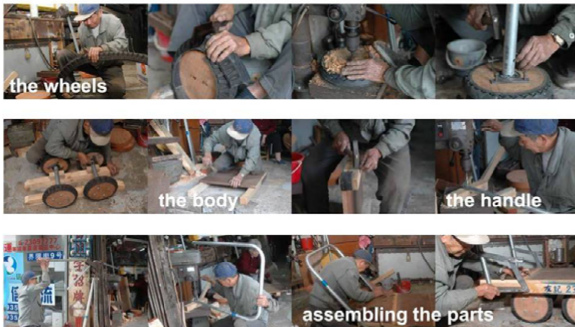
5 | A visual explication of the making process of the Yau Kee wooden cart
