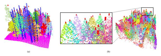
Figure 2. (a) Point cloud of a circular plot from Dataset (I), with marked tree positions from field inventory (blue bars) and manually refined tree top locations (red cylinders). (b) Manually derived tree positions marked within the point cloud of Dataset (II) by red cylinders. Point colors represent single tree clusters.
