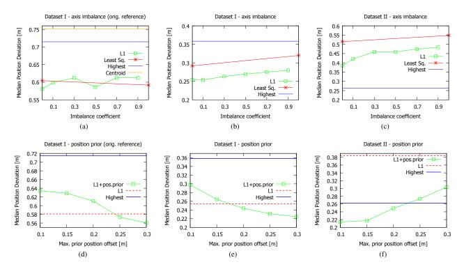
Figure 4. Median of tree position deviation as a function of maximum allowed axis imbalance (a)-(c) and maximum distance from apriori position (d)-(f). (a),(d) show result of comparison with original, unaltered measurements from field inventory, whereas (b),(c),(e),(f) are based on manually derived tree positions.
