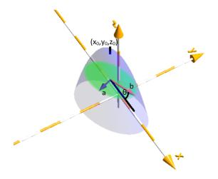
Figure 1. Z-axis aligned elliptic paraboloid centered at  $(x_0, y_0, z_0)$ , rotated by  $\theta$  degrees around the Z axis, with semiaxis lengths a, b.
