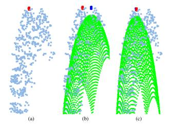
Figure 5. (a) Undersegmented point cluster with two peaks, reference position marked in red. (b) Best paraboloid fit without position prior, center marked in blue. (c) Best paraboloid fit with position prior,  $\delta=10$  cm.
