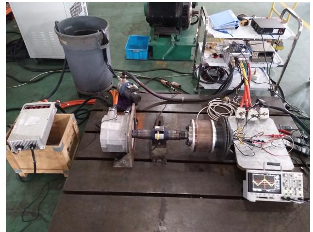
FIGURE 15. Test bench of the proposed SSDPM.
