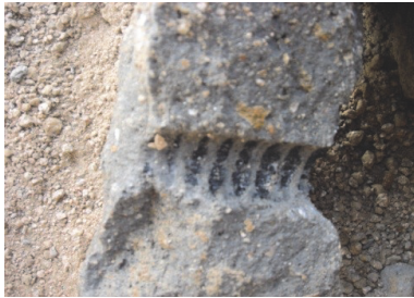
(a) Relative slippage between the anchor and anchorage bolt
