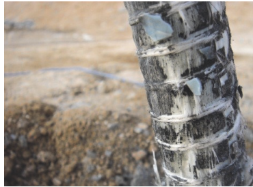
(b) Surface white-spot crack
