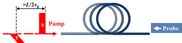
Fig. 2. The configuration of orthogonal pump pulse sequence at each scanning frequency to suppress polarization dependent fluctuation.
