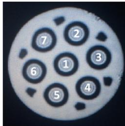
Fig. 1. Cross sectional view of the multi-core fiber used in the experiment.
