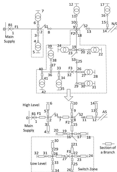
**Figure 1.** The equivalent process of a typical distribution system.
