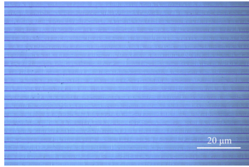
Fig. 13. Microscope image of the generated sinusoid freeform surface in a small zone.
