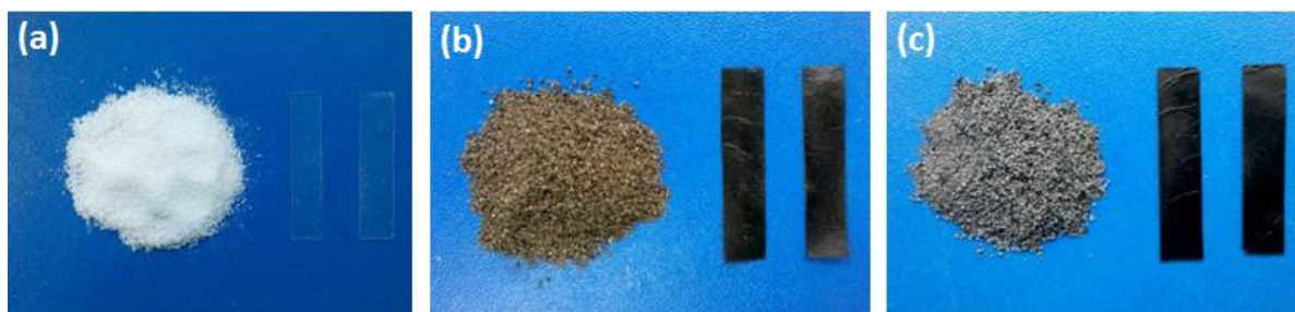
Figure 4. Original dried-powders of (a) neat PBA-PMMA, (b) GO/PBA-PMMA and (c) RGO/PBA-PMMA composites and their films processed by compression molding under 35 MPa for 5 min at room temperature.
