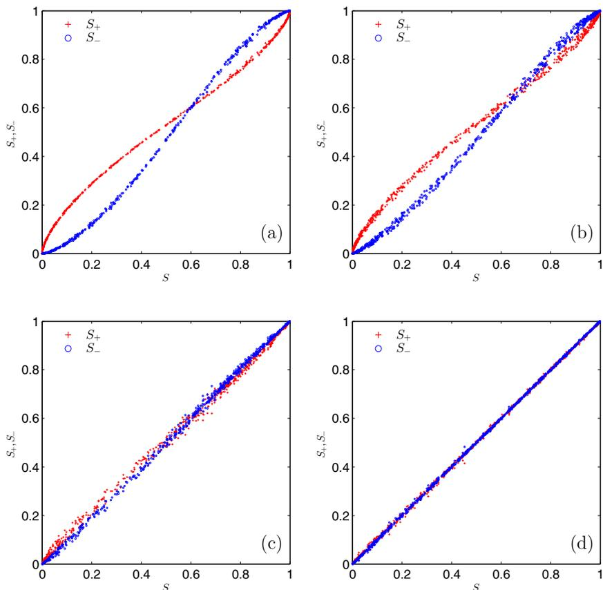
Fig. 3. Scatter of scalars at various  $x^*$  locations in the mixing layer. (a)  $x^* = 30$ ; (b)  $x^* = 60$ ; (c)  $x^* = 120$ ; (d)  $x^* = 422$ .
