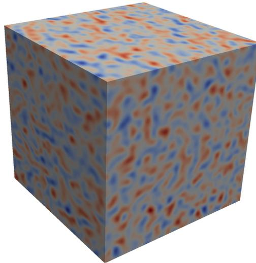
Fig. 2. Contours of initial velocity magnitude on the bounding box of the simulation domain for homogeneous isotropic turbulence.
