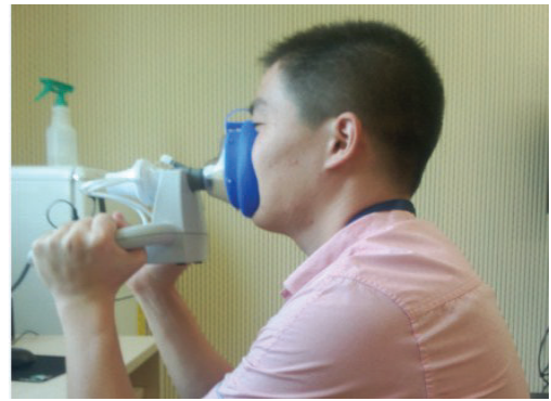
Fig. 2. The demonstration of airflow collection using PAS.
