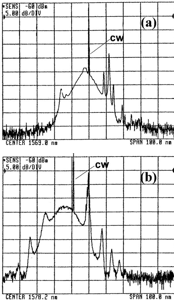
Fig. 6. Soliton spectra with coexistence of cw mode excitation and subsideband generation: (a) a case with large wavelength-shifted subsidebands; (b) a case with small wavelength-shifted subsidebands.
