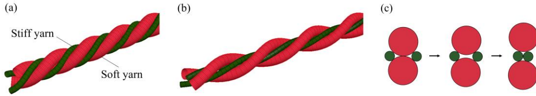
Figure 2 4-ply auxetic yarn: (a) at rest; (b) under tension; (c) at different states in cross-section view.
