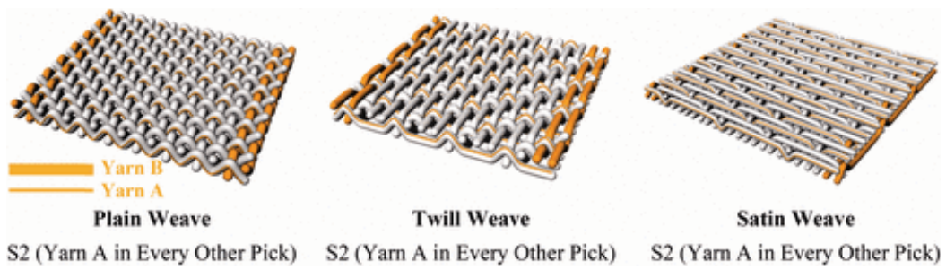
Figure 2. Three basic structures of woven fabric.
