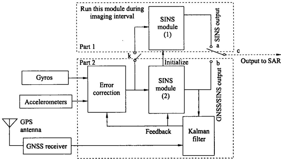
Fig. 2 Overall functional block of SAR MIS without MINS
