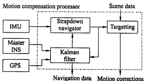
Fig. 1 Block diagram of MIS aided by MINS
